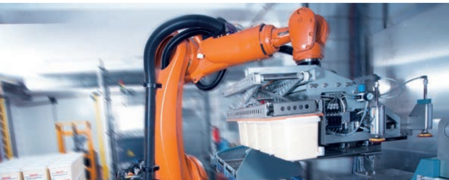
> This articulated arm robot palletizes deli salads and secures them with intermediate layers for transport.
