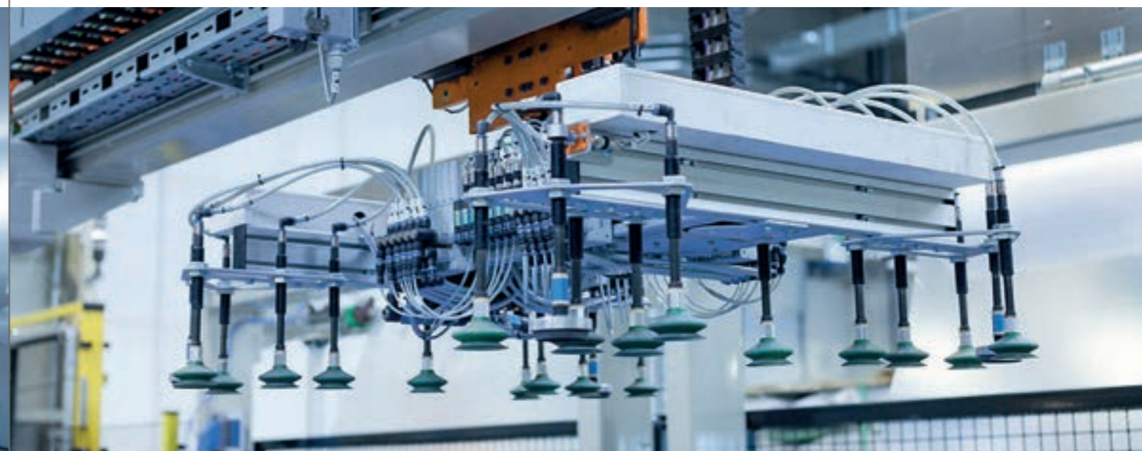
> They are our palletizing giants: portal robots that lift the heaviest weights even over long distances. They are used in the automotive industry, for example.
