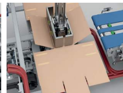
A folding matrix shapes the carton, glues and grouts the glue via stamps underneath the gantry.
