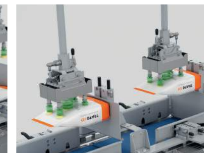
A pick and place robot (delta, gantry or kinematics) carefully picks up the products.
