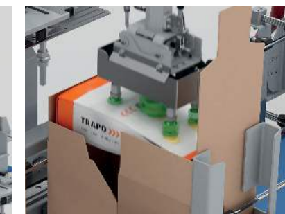
The product is kept flat, turned by 90° and put into the carton.
