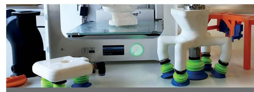
In the TRAPO technical center, components for gripper systems are developed, realized in the 3D printer and tested under real conditions.
