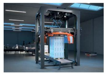
> Strong hold - low film consumption: The TRAPO Stretch Wrapper (TSW series) enables fully automatic securing of pallet loads.
