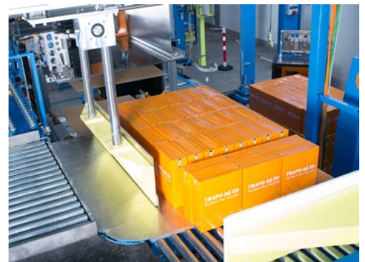
➤ A layer-slider feeds the layer of cartons precisely to the gripper.
